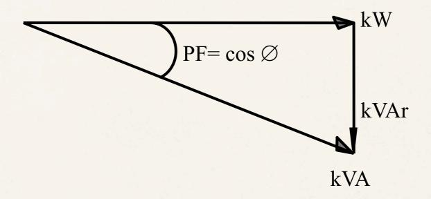
Power Factor is defined as the Real (Active) Power divided by the Apparent Power i.e. kW/kVA
