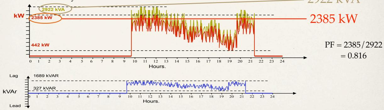
The above plot is on one of the agricultural feeder. In-operation hours are 9:30 Hrs. The plot is taken when there is no capacitive compensation provided on the feeder. Total number of APFC systems per feeder to be provided 45 No.(various ratings)
